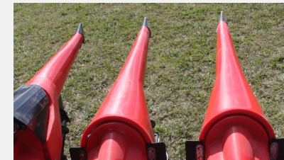
Low profile conical plastic bonnets and wide input canal for various plants between the bonnets.
