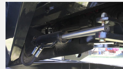
The plates that cover the rolls can be hydraulically adjusted from the combine.
