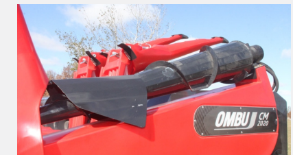
Upper side rolls helps to guide the plants. Speed rolls can be adjusted from the combine.
