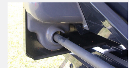
Independent auger shaft with two speeds available.
