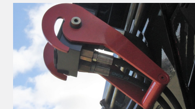
Each header has a hydraulic coupler according the brand of the combine.
