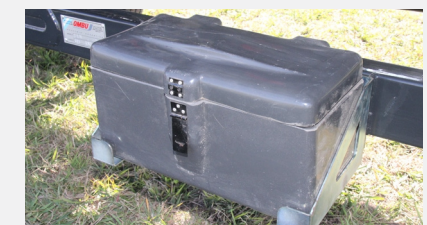
Plastic toolbox placed on the trailer beam.
