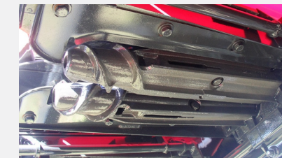
Gearbox rolls made in cast iron and placed on the gearbox output shafts. No bearing or greasing point on them.
