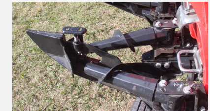
Gathering sets with front deliverers rolls turn in higher speed than the gathering chains.
