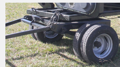
Transport trailer with turn table and matching the length of the header. Foldable draw bar.
