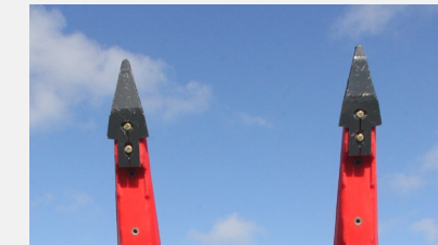
Bonnet tips made in Hardox 450 steel to resist the wasting.
